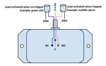
2.4.3 Note that NC and NO only have this behavior with the default polarity of 0. Their behavior will be reversed if the polarity is 1. That is, NC will be open when level and NO will be closed when level. For more information, see 4.4.
