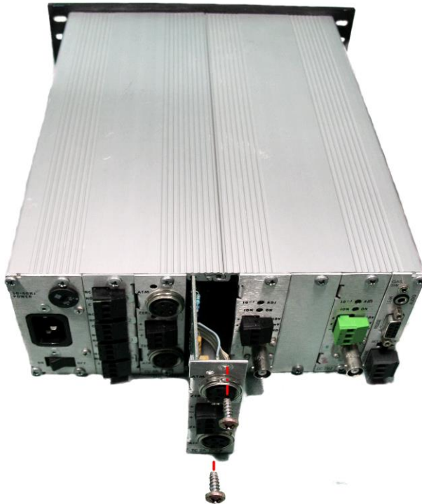
Fig. 3.3 - Removal / Installation of Modules
