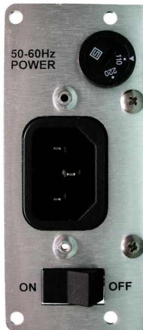
Fig. 3.4 - Power Supply Module
