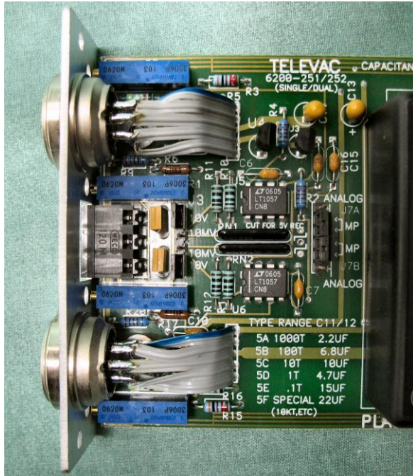
Fig. 9.6b - Capacitance Diaphragm Module Details
