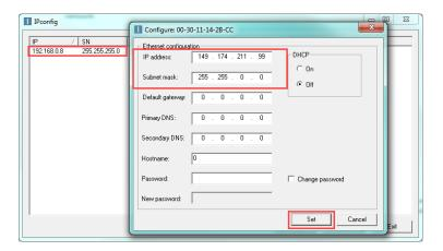
3.1.10 If DHCP is used, the IP address will be assigned automatically, but could be changed by the DHCP server. If a connection is made to a static IP address from a PLC to a device with a DHCP-assigned IP address, it will need to be verified and potentially modified before use.
