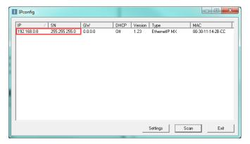
4.1.9 Select this device to change the settings. In this example, the terminal revealed in step 4.1.4 that the network needed is 149.174.211.X with a subnet mask of 255.255.0.0. The device will be set to 149.174.211.99 with a subnet mask of 255.255.0.0. This example IP address was verified to not conflict with any other devices on the local network. Once changes to the settings are complete, select Set. Select Scan to refresh the list.
