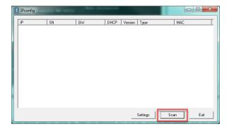
3.1.6 If the device does not show up, open the Network and Sharing Center in the Control Panel and verify that an Ethernet connection is being made. If there is no connection, check the cable and reinsert the Ethernet cable into the adapter on the computer.
