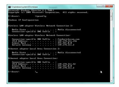
3.1.4 Find the "Ethernet adapter Local Area Connection", and mark down the IPv4 Address and Subnet Mask. This will be the network to assign to the unit. In order to communicate on the network properly, a different IP address on the network that is not in use by any other device will be needed. IT help may be needed to verify at this step; if the unit IP address conflicts with any other device on the network the unit will not communicate.
