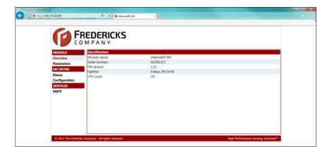
3.2.3 The unit should now be ready to use with a PLC. Please refer to Televac Application Note 3016 for downloading the Electronic Data Sheet (EDS) and creating a connection.
