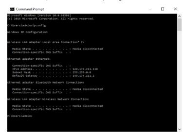
4.1.4 Find the "Ethernet adapter Ethernet", and mark down the IPv4 Address and Subnet Mask. This will be the network to assign to the unit. In order to communicate on the network properly, a different IP address on the network that is not in use by any other device will be needed. IT help may be needed to verify at this step; if the unit IP address conflicts with any other device on the network the unit will not communicate.
