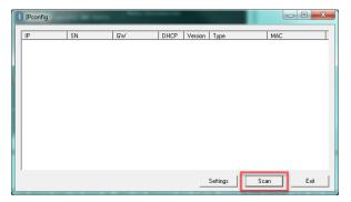
4.1.6 If the device does not show up, open the Network and Sharing Center in the Control Panel and verify that an Ethernet connection is being made. If there is no connection, check the cable and reinsert the Ethernet cable into the adapter on the computer.
