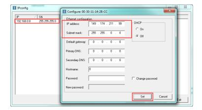
4.1.10 If DHCP is used, the IP address will be assigned automatically, but could be changed by the DHCP server. If a connection is made to a static IP address from a PLC to a device with a DHCP-assigned IP address, it will need to be verified and potentially modified before use.
