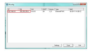
3.1.9 Select this device to change the settings. In this example, the terminal revealed in step 3.1.4 that the network needed is 149.174.211.X with a subnet mask of 255.255.0.0. The device will be set to 149.174.211.99 with a subnet mask of 255.255.0.0. This example IP address was verified to not conflict with any other devices on the local network. Once changes to the settings are complete, select Set. Select Scan to refresh the list.
